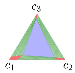
**Figure 3.1:** Thermodynamic ternary phase diagram when  $\chi_{12} = 2.5$ ,  $\chi_{13} = 3.0$ , and  $\chi_{23} = 3.5$ . Red region indicates one phase coexistence, green region indicates two-phase coexistence, and blue region indicates three-phase coexistence. Produced by Sheng Mao from Princeton University.
