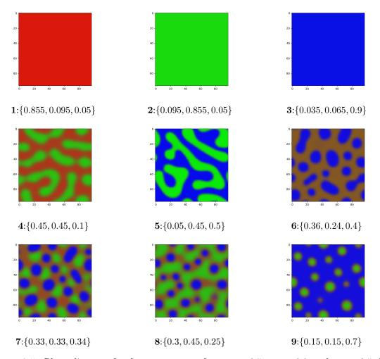
**Figure 3.5:** Phase diagrams for the ternary case when  $\chi_{12} = 2.5$ ,  $\chi_{13} = 3.0$ , and  $\chi_{23} = 3.5$  that correspond to the labels in Figure 3.3(b). Numbers in curly brackets are concentrations of  $c_1$ ,  $c_2$ , and  $c_3$ , respectively. Top row is one-phase region. Middle row is two-phase region. Bottom row is three-phase region.
