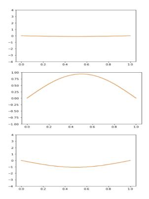
Figure 2.2: Output of using FEniCS to solve the wave equation. This output shows evolving standing wave for three subsequent time steps.
