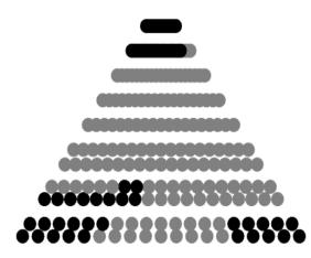
**Figure 3.6:** Kinetic ternary phase diagram created from eigenvalues of the Hessian matrix when  $\chi_{12} = 2.5$ ,  $\chi_{13} = 3.0$ , and  $\chi_{23} = 3.5$  at various compositions. The black dots indicate the concentrations that give rise to two positive eigenvalues, indicating that those correspond to one-phase coexistence. The gray dots indicate the concentrations that give rise to one positive eigenvalue, indicating that those correspond to two-phase coexistence.
