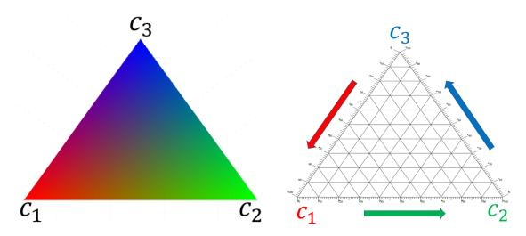
Figure 3.2: Left is a reference RGB triangle for the different components used in ternary system. Right adapted from https://commons.wikimedia.org/wiki/File:Ternary\_plot\_1.png. Arrows point toward increasing concentration on the axis of the component with the matching color.
