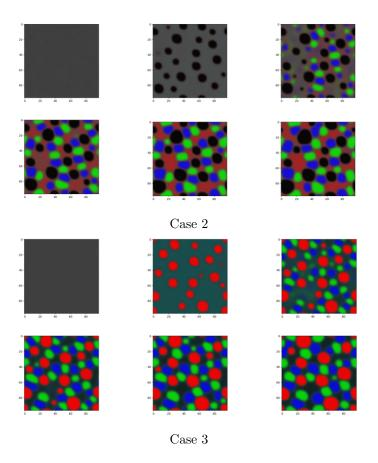
Figure 3.8: Evolution of Quaternary Cases 2 and 3 in Table 3.2. For both cases, the top row corresponds to number of time time steps: 10, 350, 700, the bottom row corresponds to number of time steps: 1000, 1500, 2000. Time step are  $10^{-4}$  seconds.
