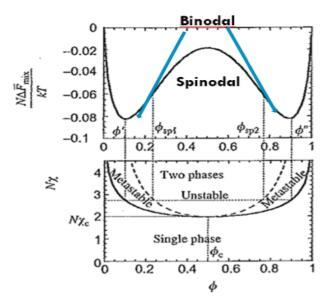
Figure 1.1: Binary Phase Diagram. Top: On x axis is the concentration of one of the components. On the y axis is the normalized free energy. Bottom: On the y axis is the value of interaction energy,  $\chi$ . Figure adapted from Reference [19].
