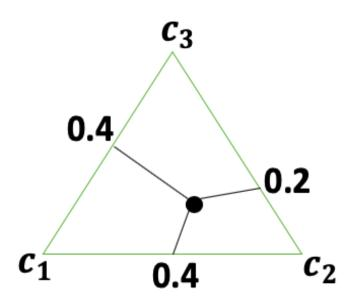
Figure 3.3: All interior points correspond to a concentration profile. In this example, the interior point corresponds to a concentration of  $0.4 c_1, 0.4 c_2$ , and  $0.2 c_3$ .
