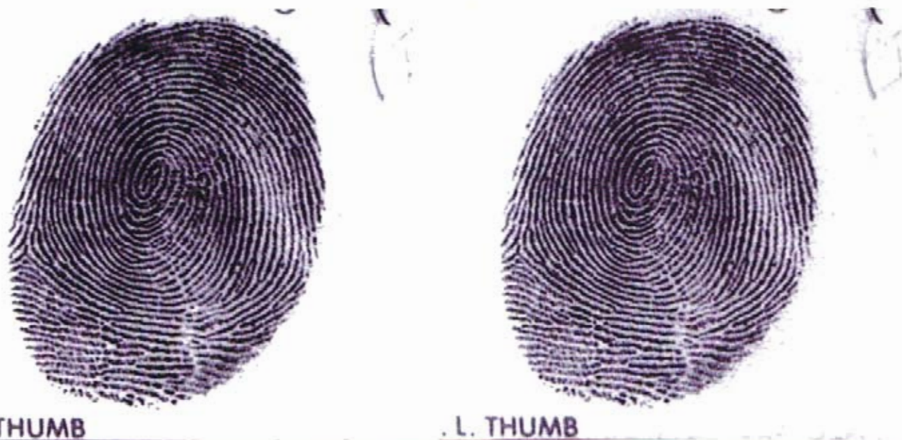
Figure 3. (Left) Original 768 \times 768 8-bit Gray-scale fingerprint image. (Right) Fingerprint image compressed 26.0:1. (Photos courtesy of Chris Brislawn, Los Alamos National Laboratory.)
