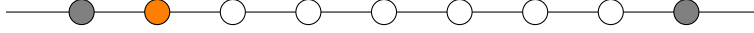
FIGURE 5. Scattering model in dimension one. The gray vertices denote sinks and the orange vertex is the source vertex for a signal entering the scattering region from the left. As per figure 4, we would like to recover what exits the system at the right end of the region, at the rightmost gray vertex.
